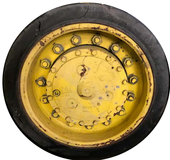
Example of a tire that is cracked and worn and needs replacing.
