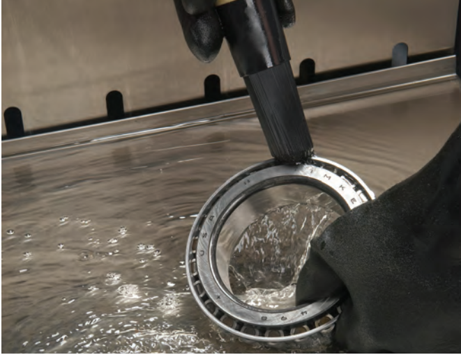
Fig. 3. Smaller bearings can be cleaned in a wash tank.
