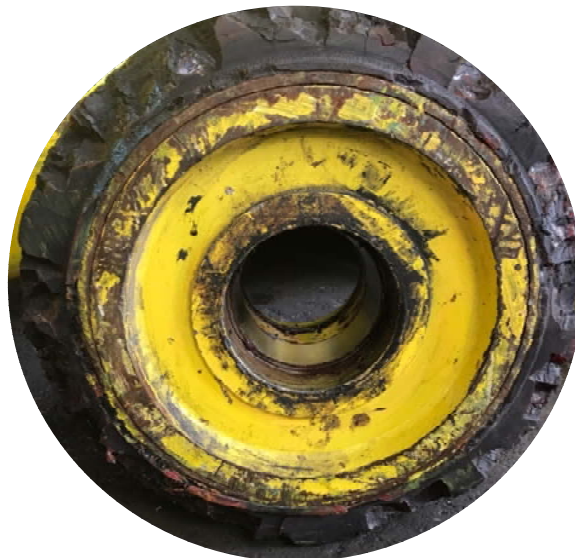
Example of a tire that is severely chunked and needs replacing.
