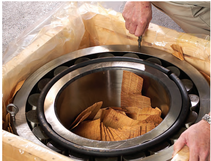
Fig. 2. Eyebolts can be inserted into lifting holes.
